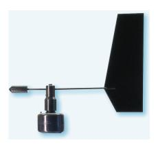
Light weight, long life potentiometer vane. Mechanical angle  $360^\circ$  without stop. Electrical angle  $350^\circ \pm 3^\circ$ , threshold is between 1.2 and 1.5 m/s. The PRV is an affordable high quality wind vane with oil bronze bearings and stainless steel mounting hardware.
