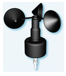
Light weight cup anemometer based on Hall effect principle. Measuring range 0..60 m/s with a treshold of 0,5 m/s. Two pulses per rotation and 67 pulses at 30 m/s. The PA2 is an affordable high quality cup anemometer with ceramic magnets and stainless steel bearings and mounting hardware.
